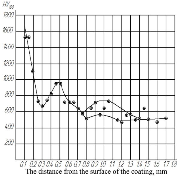
Fig. 3. The microhardness values in depth of hard-alloyed coating obtained by molding with the insert in the model of thickness 2,0 mm, after quenching at a heating temperature of 1150<sup>0</sup>S and tempering 200<sup>0</sup>S.
