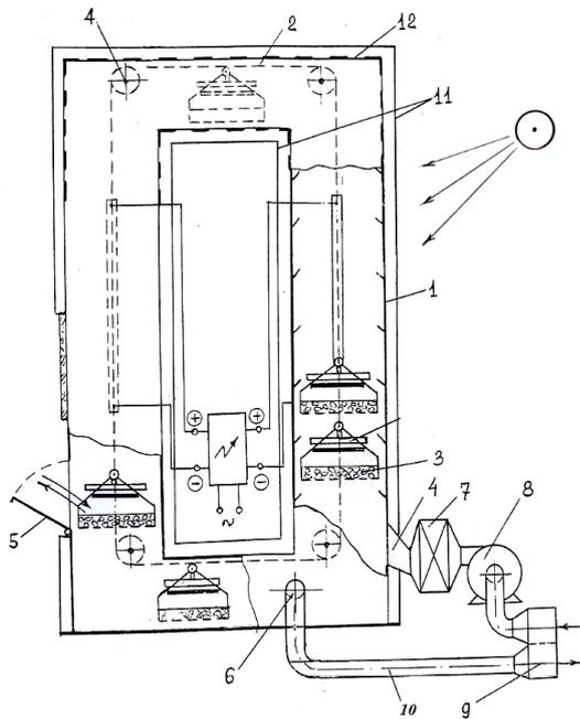
Fig. 1. Principle scheme of vertical cradle-conveyer type solar-fuel drying installation
