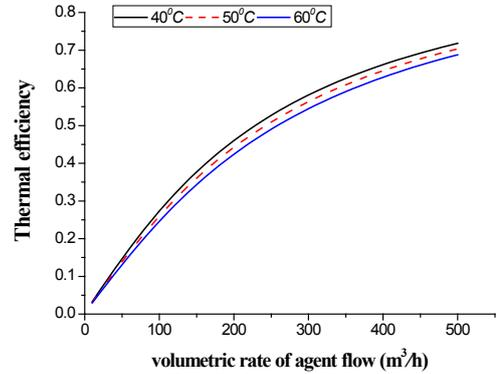
Fig. 3. The dependence of thermal efficiency of  $\eta_{te} = f(L)$  on L – volumetric rate of agent flow
