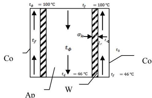
Fig. 2. A principal scheme of thermal balance components of solar collector
