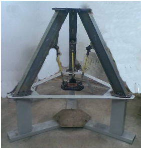
a) - frame layout three coordinate drill-mill machine-tool with MPS [7]
